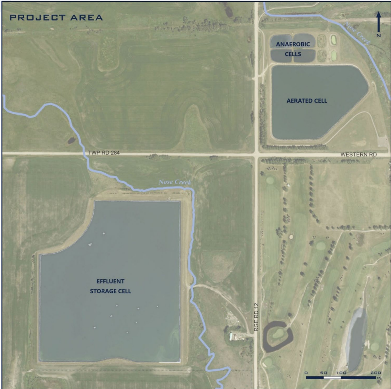
Figure 2.2: Satellite Image of the Town of Crossfield's WWTF
