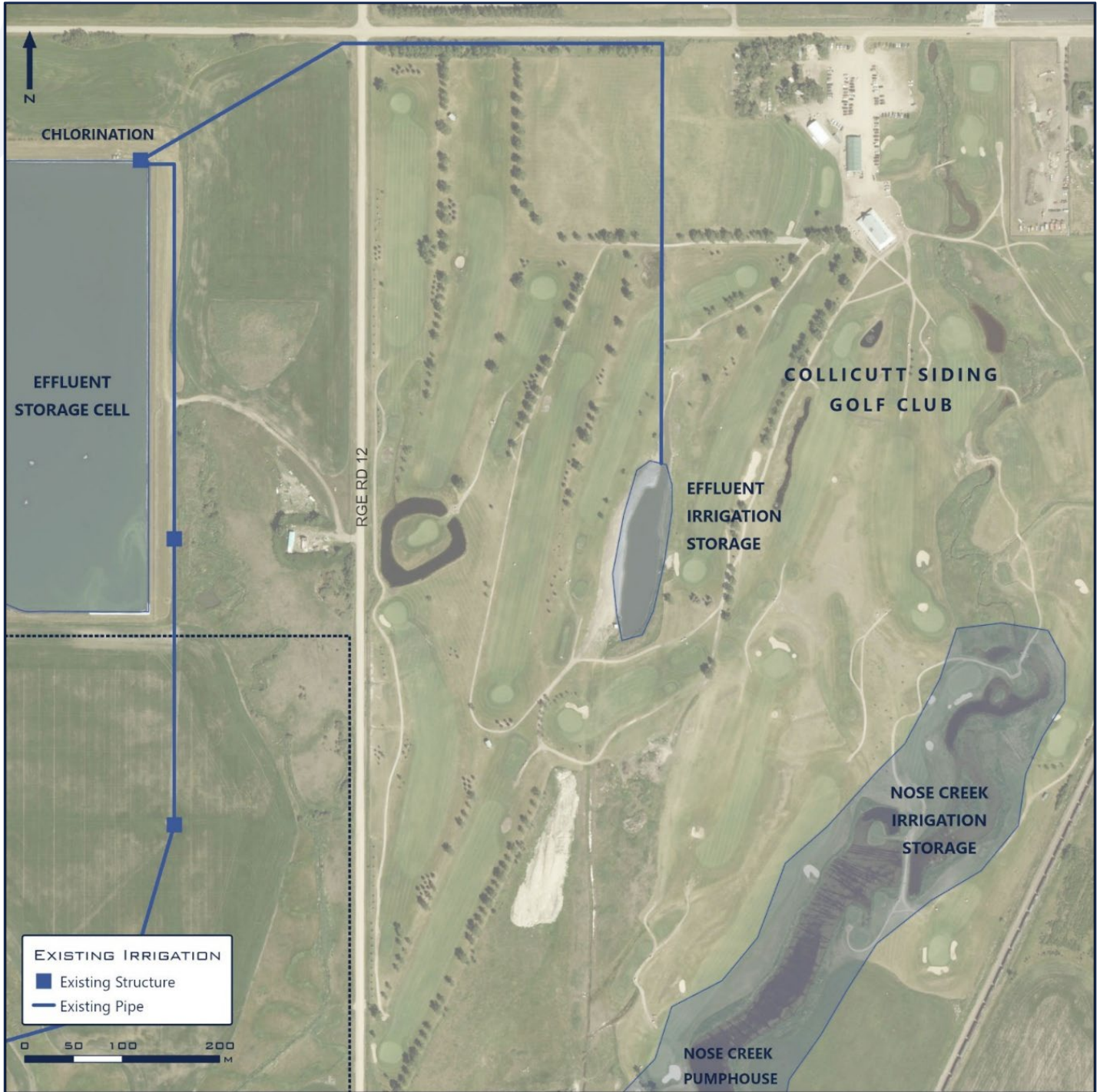
Figure 2.6: Existing Collicutt Golf Course Irrigation Layout
