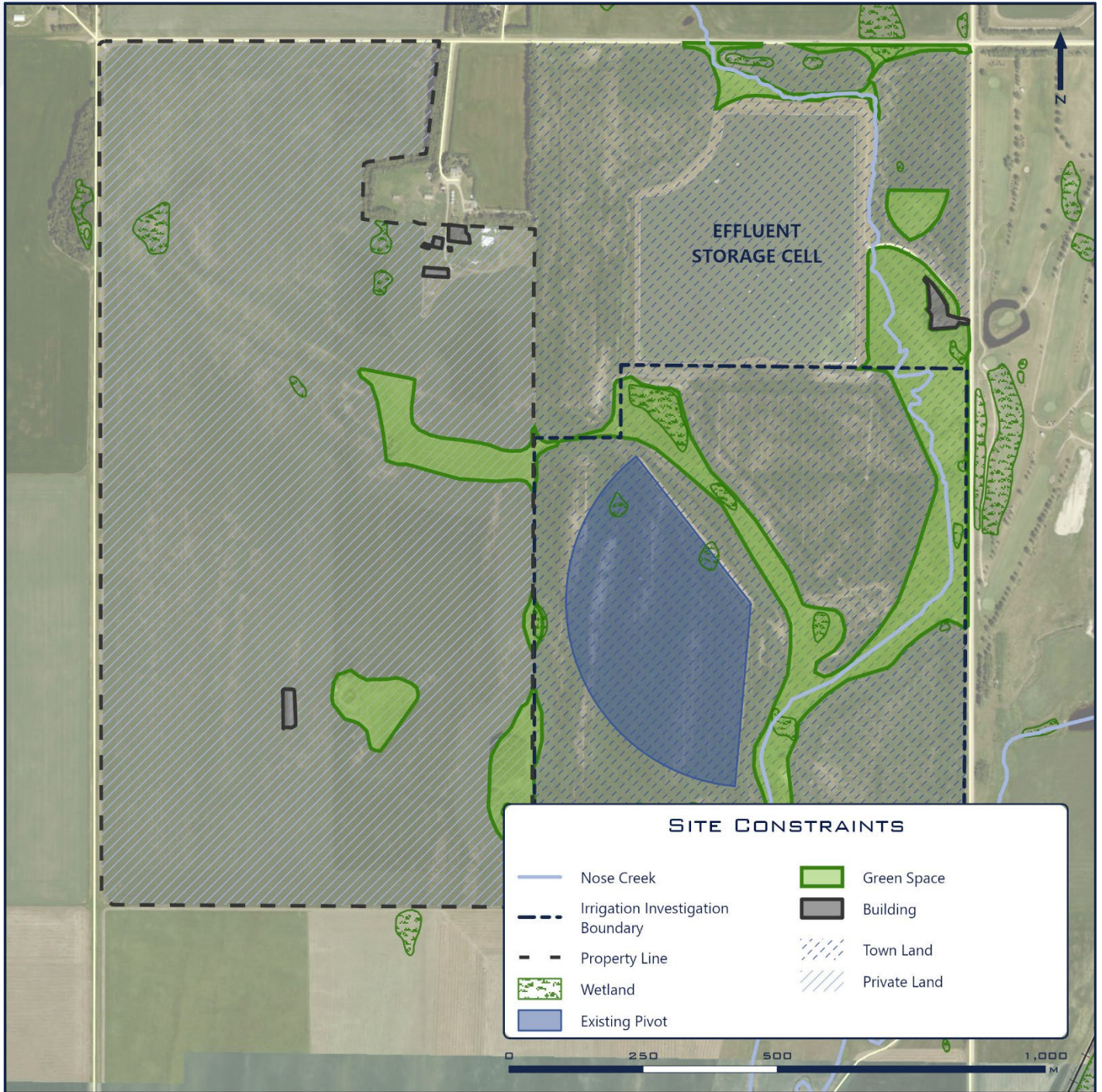
Figure 2.3: Site Review for Potential Irrigation and Treatment Wetland
